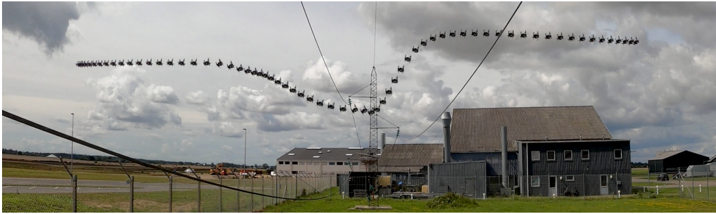
(a) Power lines are avoided (left to right) while flying at upwards of 10 m/s. The top wire is 10 mm in diameter, while the bottom three conductors are 20 mm in diameter. The shortest distance between the power lines is about 3 meters.
