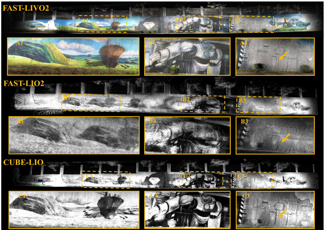
Fig. 7. Comparison of mapping results on the HIT Graffiti Wall sequence: Top : FAST-LIVO2, Middle : FAST-LIO2, Bottom : CUBE-LIO. CUBE-LIO provides sharper, less ghosted structures.
