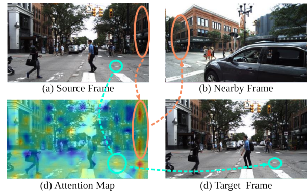
Fig. 9. Visualization of attention map on DDAD [16] dataset. It can be observed that the attention module highlights certain key areas, which contribute to the estimation of scale information and the pose transformation estimation between adjacent frames.
