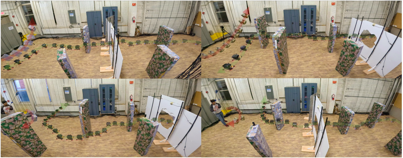
Fig. 4. Sequence of images of quadrotor navigating through different scenarios. Green and red arrow shows the path of the robot and the dynamic obstacle respectively.
