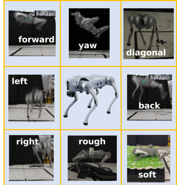
Fig. 1: Versatile jumping experiments conducted on Unitree-Go2, including omnidirectional jumping and landing on different terrains.
