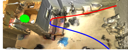
Fig. 2: Example of 2 separate classical reactive planning runs, depicted in red and blue, getting stuck in the same local minimum. The goal location is behind the wall, depicted in green. BundleFusion dataset [1].
