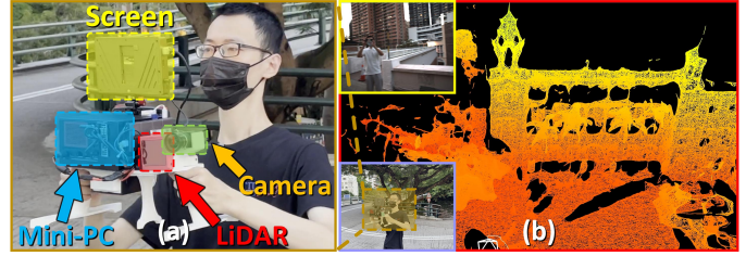
Fig. 6: (a) shows our handheld device for data collection and online mesh reconstruction. (b) shows a snapshot of our accompanying video [70] (starting at 00:09) of Experiment-1, with three time-aligned views of different sources including a screen-recorded view (in red), a camera preview (in yellow), and a third-person view (in blue).
