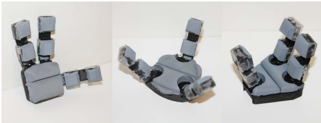
Fig. 5. Our ROMEO fingers and three different passively double compliant palm configurations. From left to right, we have an anthropomorphic, a 120°, and a “Y” configuration gripper.
