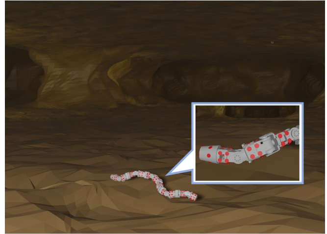
Fig. 1: Snake robot with whole-body tactile sensors performing cave navigation.
