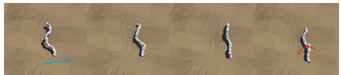
Fig. 15: Tactile-less CPG controller has difficulty traversing the terrain with sidewinding gait, the robot falls from uphill climbing.
