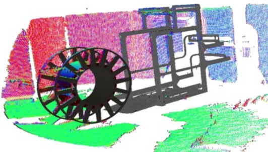
Fig. 8: Example of multi-object tracking: bobbin and unwinder. The colors illustrate the normals estimated from the captured point cloud. The grey parts correspond to the models.
