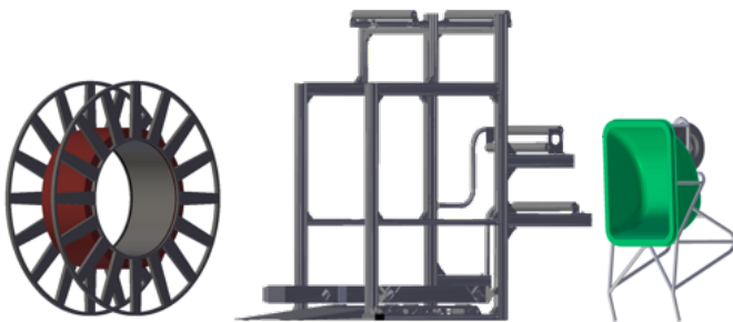
Fig. 5: 3D model of the bobbin, a simplified unwinder and a wheelbarrow. The bobbin and unwinder (real and models) are provided by an industrial partner.
