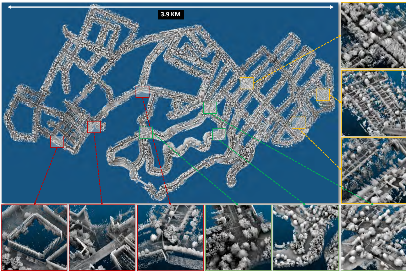
Fig. 11. Offline Merging on the Pittsburgh Dataset. The above map is merged using 43 retrieved segments with limited overlaps from the Pittsburgh dataset. We show examples of open-street areas (bounded in red), terrain areas (bounded in green), and residential areas (bounded in yellow).
