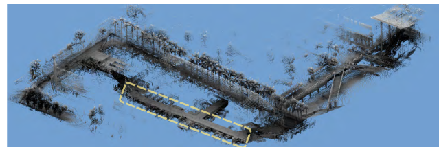
a) The merged map for three trajectories sharing overlapped areas in an underground passage.
