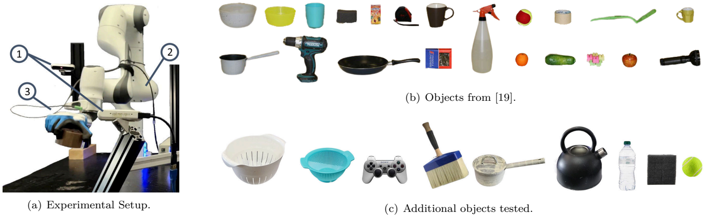
Fig. 9. Experimental setup and complete set used for the experimental validation (a). 30 objects, of which 21 are the ones used in [19] (b) and 9 additional objects (c), from left to right: Big Colander, Small Colander, Controller, Brush, Pot, Boiler, Bottle, Foam Brick, Tennis Ball.
