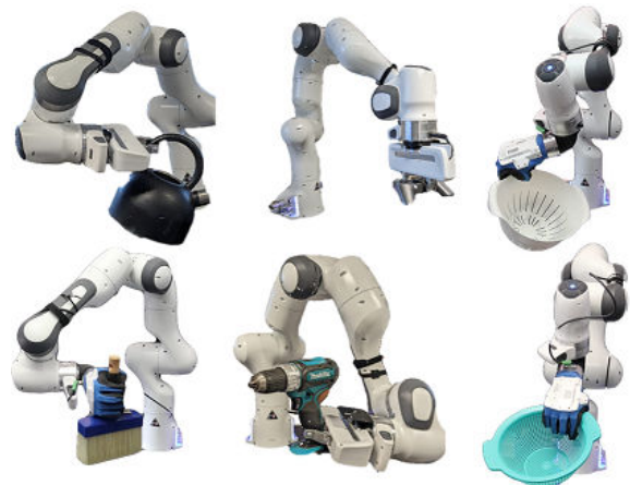
Fig. 1. The ability to grasp previously unseen objects with different grippers, adapting to imperfectly known, highly dynamic, and unstructured situations is crucial to enable general-purpose robots to be effective in a large field of use cases.
