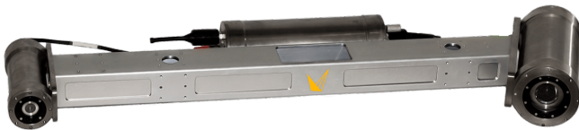
Fig. 4: An Insight Pro underwater laser scanner developed by Voyis Imaging Inc. The beam emitter is on the left, while the camera is on the right. 3D point clouds are produced by triangulating the laser beam. The baseline between the emitter and the camera is approximately 1 m.
