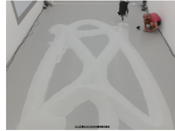
Fig. 11. The structure after the deposit of 1.7 tons of powder.
